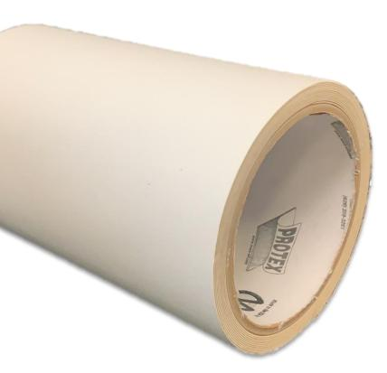
PROTEX 20S is a 20 mil latex saturated paper designed for applications where extra protection is needed, and high tack is required. PROTEX 20S has proven to be excellent in protecting graphite composite surfaces and tooling from impact damage that may result in possible interlayer fracturing. PROTEX 20S is also used for movie studio backdrops, cover-ups and painting of sets. It can withstand 60 lbs. of sandblasting pressure for decorative applications e.g., glass etching, and light sandblasting.
